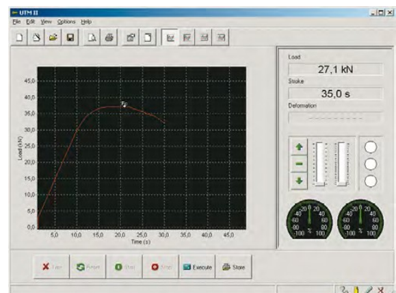
MG030-01 Software remote control from PC
