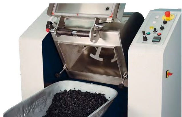
Easy tilting with rotation angle up to 130°
