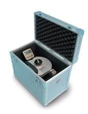
Compact, light, for use in any location, this Pull-Off Tester is fitted with a load cell and high resolution large digital display unit; it is therefore suitable for measurements from low loads up to 16 kN, granting a wide working range and ideal for a large number of applications and materials. The direct tensile force is applied by rotating the hand wheel.
