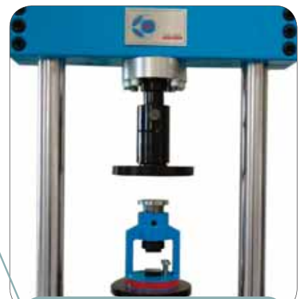
Cement compression test
