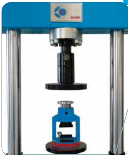
Cement bending test
